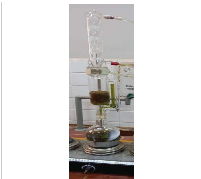
Figure 1: Soxhlet- prepare the hot ethanol extract of the Artemisia herba-alba .
